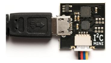
I<sup>2</sup>CMini also has a micro USB connector. Its Qwiic connector is polarized; it attaches as shown. The color coding for the signals is the same as for I<sup>2</sup>CDriver.
